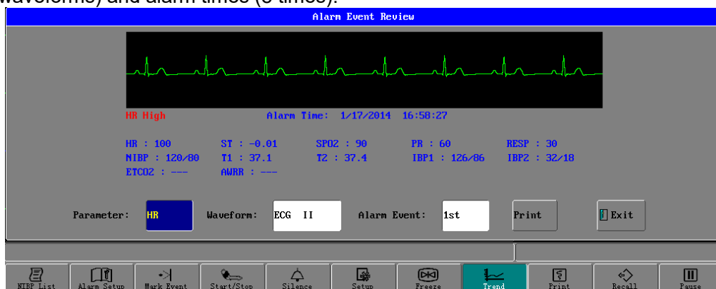
Figure 31: Window for Alarm Event Review
