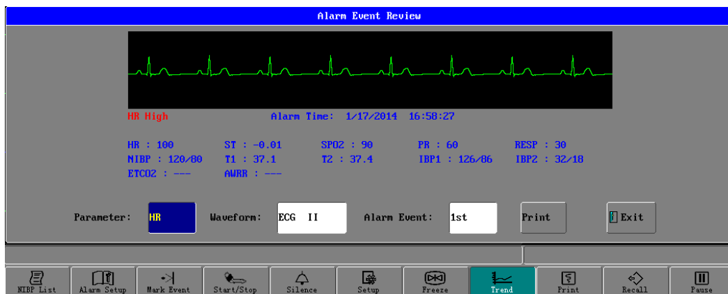
Figure 355: Window for Alarm Event Review
